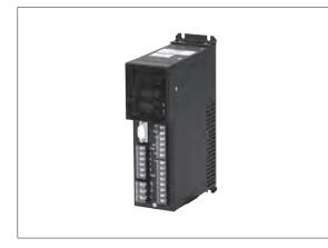
In the DC-A2M controller, the functions for inputting and displaying the settings required for controlling digital valves and for driving the valves have been completely integrated. This controller can be used for all digital valve models which incorporate a 2-phase motor.
