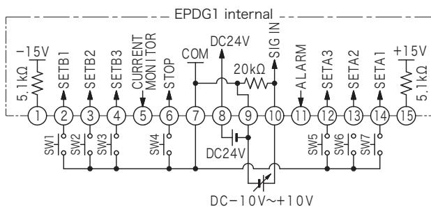
Flow output set by SETB1 VR when SW1 is ON.
