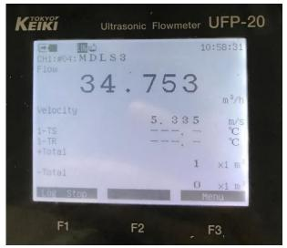
As demonstrated in applications such as this, the portable UFP-20 flowmeter used in combination with a variety of sensors can successfully measure pipes with nominal diameters from 13mm - 5000mm.
