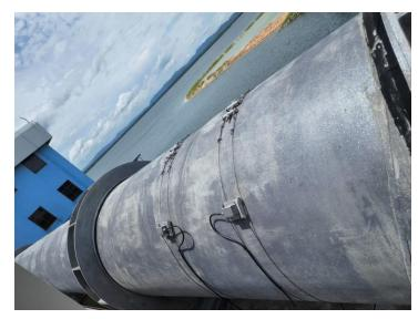
The UFL-30 series stationary, clamp-on ultrasonic flowmeter with multi-path measurement capability incorporating up to 4 pairs of transducers placed on the outside of pipes provides stable instantaneous flow rate measurements.
