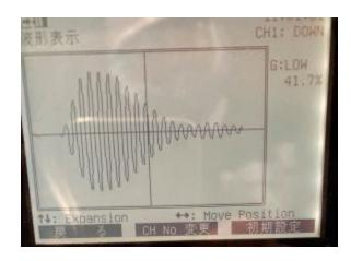
As verification test at site such as above photo, the portable UFP-20 flowmeter used in combination with large transducer successfully which can measure pipes with nominal diameters from 300mm up to 5000mm.
