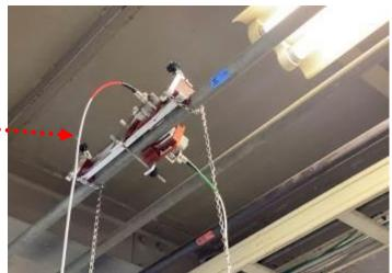
The UFP-20 portable, clamp-on ultrasonic flowmeter provides instantaneous flow rate measurements with up to 2 pairs of transducers placed on the outside of pipes.
