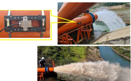
The "Intelligent digital UFW-100" stationary, clamp-on ultrasonic flowmeter with transducers placed on the outside of pipes provides stable instantaneous flow rate measurements.
