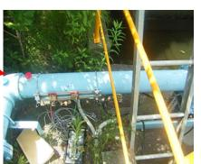
The UFP-20 portable, clamp-on ultrasonic flowmeter provides instantaneous flow rate measurements with up to 2 pairs of transducers placed on the outside of pipes.
