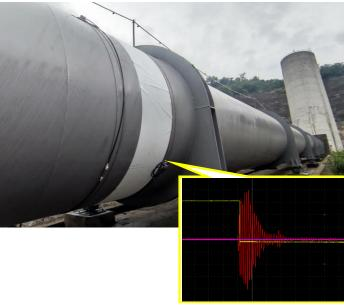
The clamp-on type ultrasonic is the best solution to be installed without stopping water or cutting pipe. Only approx. half size of pipe diameter will be required to install transducers.
