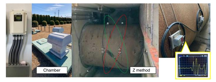
The UFL-30 series stationary, clamp-on ultrasonic flowmeter with multi-path measurement capability incorporating up to 4 pairs of transducers placed on the outside of pipes provides stable instantaneous flow rate measurements.
