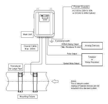
By employing the UFL-30 series stationary clamp-on ultrasonic flowmeter in combination with the appropriate sensor from the variety available and/or the system's multi-path measurement capability. You may be able to obtain high stable flow measurements of pipes from 25mm up to 6000mm in nominal diameter under less than ideal conditions.
