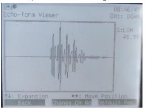
As verification test at site such as above photo, the portable UFP-20 flowmeter used in combination with 3 different transducers successfully which can measure pipes with nominal diameters from 13mm up to 5000mm.
