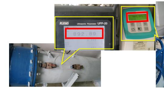
The UFP-20 portable, clamp-on ultrasonic flowmeter provides instantaneous flow rate measurements with up to 2 pairs of transducers placed on the outside of pipes.
