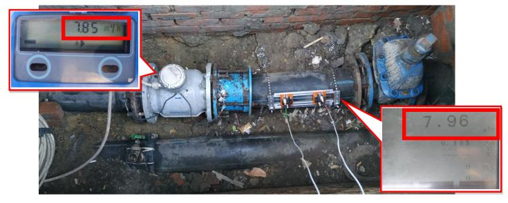
The UFP-20 portable, clamp-on ultrasonic flowmeter provides instantaneous flow rate measurements with up to 2 pairs of transducers placed on the outside of pipes.
