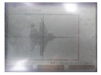
As verification test at site such as above photo, the portable UFP-20 flowmeter used in combination with large transducer successfully which can measure pipes with nominal diameters from 300mm up to 5000mm. In this case, deviation between existing flowmeter and portable was only <u>1.4%</u>.
