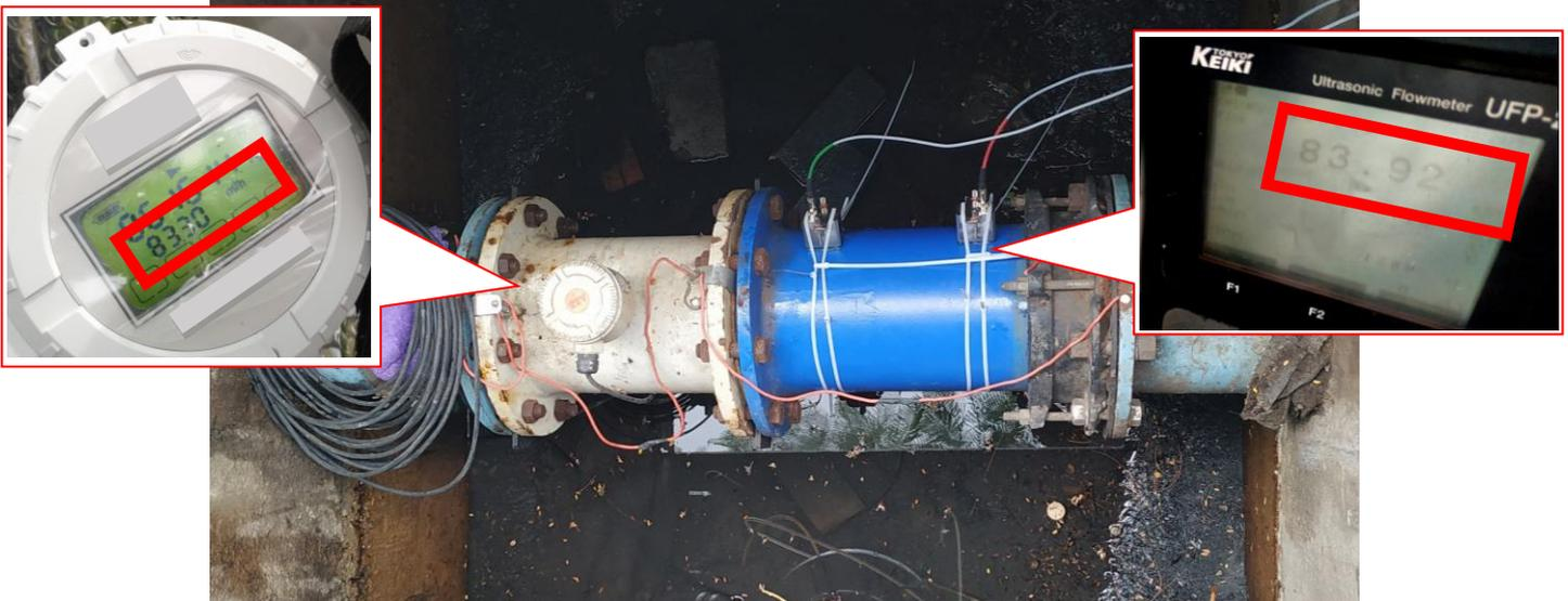
The UFP-20 portable, clamp-on ultrasonic flowmeter provides instantaneous flow rate measurements with up to 2 pairs of transducers placed on the outside of pipes.
