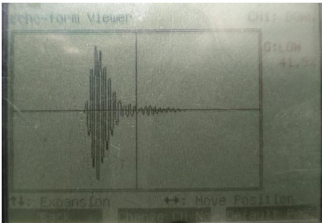
As verification test at site such as above photo, the portable UFP-20 flowmeter used in combination with large transducer successfully which can measure pipes with nominal diameters from 300mm up to 5000mm. In this case, deviation between existing flowmeter and portable was only **0.7%**.
