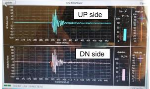
By employing the UFW-100 stationary clamp-on ultrasonic flowmeter in combination with the easy set-up function on the Windows-based graphical & user-friendly PC interface is easy to configure through such as "Wizard-parameter input", "Echo-wave check & monitoring (as above
