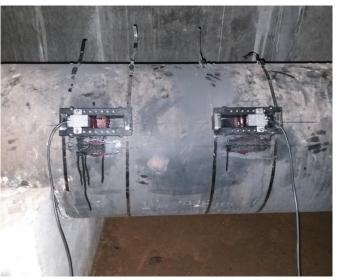
indicated) ", "Auto-Logging function", "Analog input" and / or "Integrated mounting fixture". Through such easy setup function, you may be able to obtain high accuracy flow measurements of pipes from 25mm up to 600mm in nominal diameter with±30m/s velocity range coverage.
