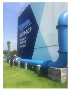
As verification test at site such as above photo, the portable UFP-20 flowmeter used in combination with large transducer successfully which can measure pipes with nominal diameters from 300mm up to 5000mm.
