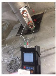
The UFP-20 portable, clamp-on ultrasonic flowmeter provides instantaneous flow rate measurements with up to 2 pairs of transducers placed on the outside of pipes.
