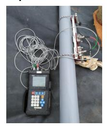
The UFP-20 portable, clamp-on ultrasonic flowmeter provides instantaneous flow rate measurements with up to 2 pairs of transducers placed on the outside of pipes.
