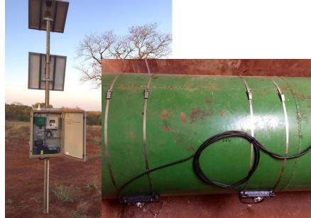
The "Intelligent digital UFW-100" stationary, clamp-on ultrasonic flowmeter with transducers placed onto the outside of pipes provides stable instantaneous flow rate measurements.
