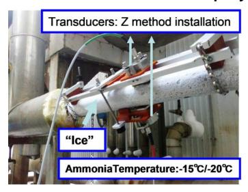
The UFP-20 portable, clamp-on ultrasonic flowmeter provides instantaneous flow rate measurements with up to 2 pairs of transducers placed on the outside of pipes.
