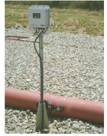
The "Intelligent digital UFW-100" stationary, clamp-on ultrasonic flowmeter with transducers placed on the outside of pipes provides stable instantaneous flow rate measurements.
