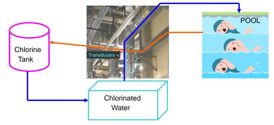
The UFP-20 portable, clamp-on ultrasonic flowmeter provides instantaneous flow rate measurements with up to 2 pairs of transducers placed on the outside of pipes.
