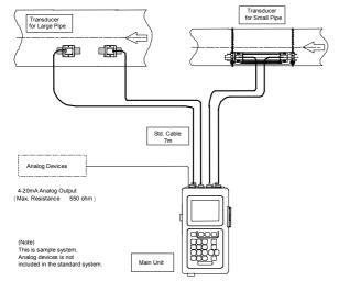
In the application of energy audit and/or ESCO, the client hopes to measure heat energy at 2 different systems or 2 different circuits in a system in the same time.
