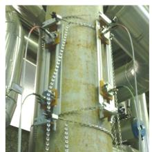
The UFP-20 portable, clamp-on ultrasonic flowmeter provides 2path measurement by 2 pairs of transducers at the measuring point that has sever flow condition.
