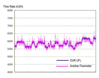
Multi-path measurement is a feature of our UFL-20 series stationary clamp-on ultrasonic flowmeter. By employing the UFL-20 series stationary clamp-on ultrasonic flowmeter in combination with the appropriate sensor from the variety available and/or the system's multi-path measurement capability. You may be able to obtain high stable flow measurements of pipes from 25mm up to 6000mm in nominal diameter under less than ideal conditions.
