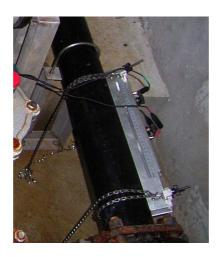
The UFP-10 portable, clamp-on ultrasonic flowmeter provides instantaneous flow rate measurements with 1 pair of transducers placed on the outside of pipes.
