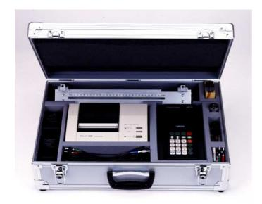
At this particular site, the UFP-10 portable flowmeter with 1 pair of sensors measured the flow rate through a 150 mm diameter pipe, non-intrusively, from the outside with no interference of flow.
