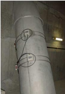
The UFL-20 series stationary, clamp-on ultrasonic flowmeter with multi-path measurement capability incorporating up to 4 pairs of transducers placed on the outside of pipes provides stable instantaneous flow rate measurements
