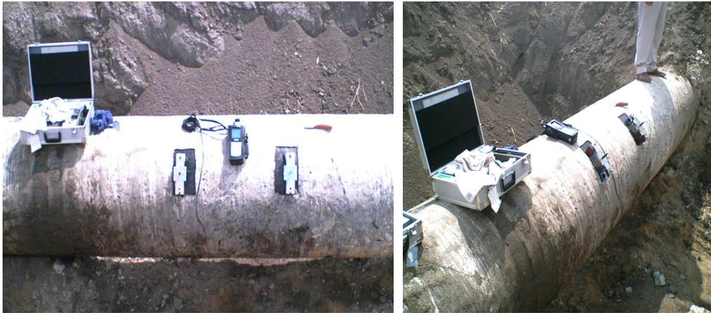
The UFP-10 portable, clamp-on ultrasonic flowmeter provides instantaneous flow rate measurements with 1 pair of transducers placed on the outside of pipes.
