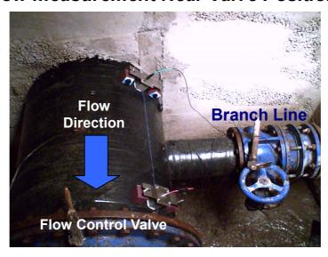
The UFP-10 portable, clamp-on ultrasonic flowmeter provides instantaneous flow rate measurements with 1 pair of transducers placed on the outside of pipes.
