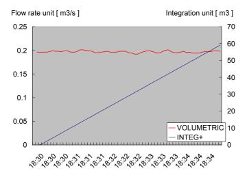
As demonstrated in applications such as this, the portable UFP-10 flowmeter used in combination with a variety of sensors can successfully measure pipes with nominal diameters from 13mm - 5000mm. The main unit's inner memory can provide long term storage (logging) of instantaneous flow rates and integral data - digital data which can then be transferred to PC's and modified for statistical analysis and other purposes.
