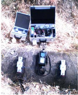
The UFP-10 portable, clamp-on ultrasonic flowmeter provides instantaneous flow rate measurements with 1 pair of transducers placed on the outside of pipes.
