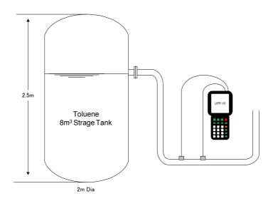
The UFP-10 portable, clamp-on ultrasonic flowmeter provides instantaneous flow rate measurements with 1 pair of transducers placed on the outside of pipes.
