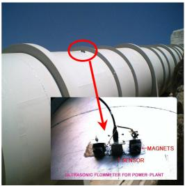
The UFP-10 portable, clamp-on ultrasonic flowmeter provides instantaneous flow rate measurements with 1 pair of transducers placed on the outside of pipes.
