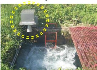
The MRG-10 micropower impulse radar level gauge features accurate, non-contact, level measurement with simple installation over a target fluid, in this case, river waters.
