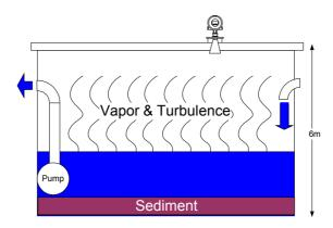
The MRG-10 micropower impulse radar level gauge features accurate, non-contact, level measurement with simple installation over a target fluid.
