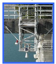
The MRG-10 micropower impulse radar level gauge features accurate, non-contact, level measurement with simple installation over a target fluid, in this case, river waters.
