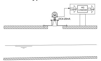
The MRG-10 micropower impulse radar level gauge features accurate, non-contact, level measurement with simple installation over a target fluid. It is incorporated in this channel water flow measurement system application to insure stable measurement of water level, unaffected by atmospherics.
