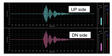
By employing the UFW-100 stationary clamp-on ultrasonic flowmeter in combination with the easy set-up function on the Windows-based graphical & user-friendly PC interface is easy to configure through such as "Wizard-parameter input", "Echo-wave check & monitoring (as above
