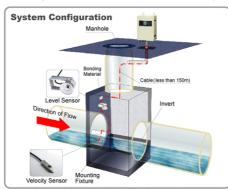
Only 1 pc of ultrasonic transducer can measures flow-velocity by pulse-doppler principle. 1 set of level gauge measures height of fluid surface. Then actual cross-section is calculated from predefined channel dimension and fluid height. Flow volume will be led as multiplied by velocity and fluid height. When water-level goes down to velocity transducer height, then automatically UVH-2000 will switch to HQ calculation mode.
