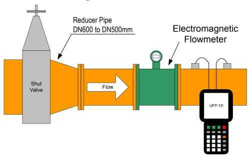
The UFP-10 portable, clamp-on ultrasonic flowmeter provides instantaneous flow rate measurements with 1 pair of transducers placed on the outside of pipes.
