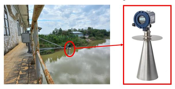
The MD-10 micropower impulse radar level gauge features accurate, non-contact, level measurement with simple installation over a target fluid, in this case, river waters.
