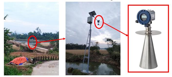
The MD-10 micropower impulse radar level gauge features accurate, non-contact, level measurement with simple installation over a target fluid, in this case, river waters.
