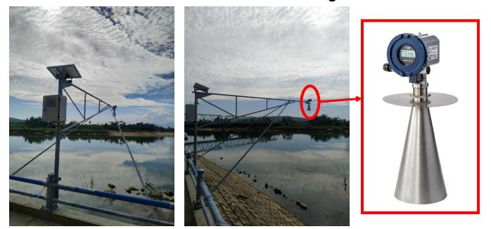
The MD-10 micropower impulse radar level gauge features accurate, non-contact, level measurement with simple installation over a target fluid, in this case, river waters.
