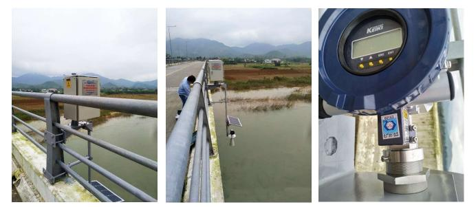
The MD-10 micropower impulse radar level gauge features accurate, non-contact, level measurement with simple installation over a target fluid, in this case, river waters.
