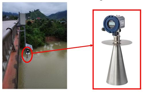
The MD-10 micropower impulse radar level gauge features accurate, non-contact, level measurement with simple installation over a target fluid, in this case, river waters.
