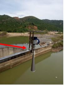
The KRG-10 radar level gauge features accurate, non-contact level measurement with simple installation over a target fluid, in this case, river raw waters.
