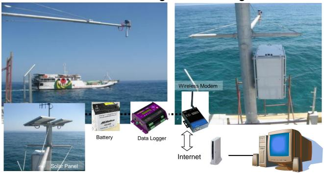
The KRG-10 Non-contacting Radar level gauge features accurate & non-contact level measurement with simple installation over a target liquid, in this case, sea surface.
