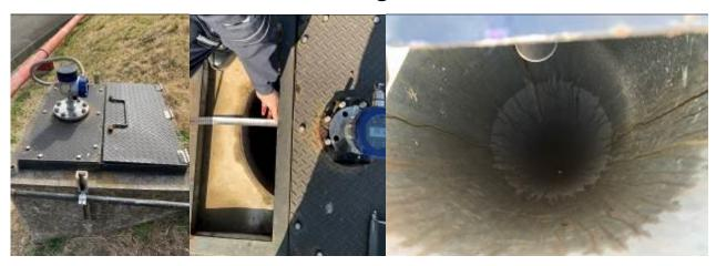
The KRG-10 radar level gauge features accurate, non-contact, level measurement with simple installation over a target fluid. In applications such as solid or powder process tanks where the sensing elements of contact type level instruments are exposed to stuck and substance adhesion, non-contact means of measurement which are unencumbered by such concerns are preferable for durability and reliability of measurement.
