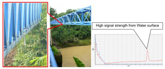
The KRG-10 Non-contacting Radar level gauge features accurate & non-contact level measurement with simple installation over a target liquid, in this case, river water surface.
