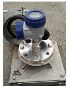
The KRG-10 micropower impulse radar level gauge features accurate, non-contact, level measurement with simple installation over a target fluid.
