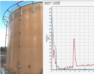
The KRG-10 radar level gauge features accurate, non-contact, level measurement with simple installation over a target fluid. In applications such as acid process liquid tanks where the sensing elements of contact type level instruments are exposed to corrosion and substance adhesion, non-contact means of measurement which are unencumbered by such concerns are preferable for durability and reliability of measurement.
