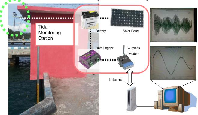
The KRG-10 Non-contacting Radar level gauge features accurate & non-contact level measurement with simple installation over a target liquid, in this case, sea surface.
