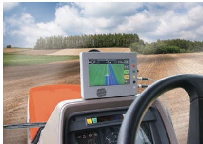
Automated straight-line assistance device for agricultural vehicles
