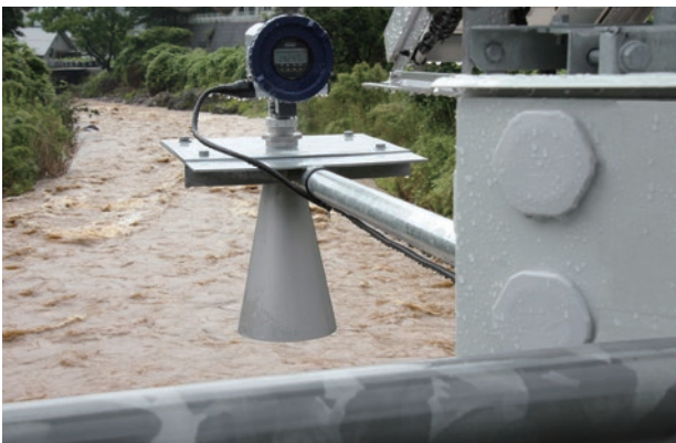
MD-10 microwave level gauge for crisis management water gauges
